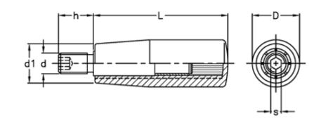
$\begin{array}{ll} D &= 22 \\ d1 &= 18 \\ d \ 6g = M6 \\ h &= 13 \\ L &= 56 \\ s &= 3 \end{array}$
